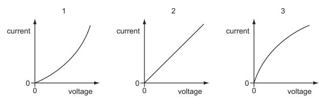
Which graph is for a resistor at constant temperature and which is for a filament lamp?
