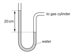
The density of water is  $1000 \,\mathrm{kg/m^3}$  and the gravitational field strength g is  $10 \,\mathrm{N/kg}$ .
